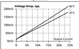
Fig. 18-3 Power losses when only one input is used
