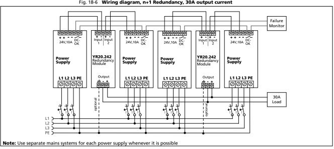
Fig. 18-6 Wiring diagram, n+1 Redundancy, 30A output current
