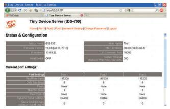
is operating abnormally, or if there is no communication between the tDS-700 and the host for a predefined period of time (system timeout). This is an important feature that ensures the tDS operates continuously, even in harsh environments.
