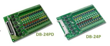
to sense a wide range of AC signals. You can also use this board to isolate the computer from large common-mode voltage, ground loops and transient voltage spikes that often occur in industrial environments, as illustrated below. Table A4-1 is the comparison of DB-24P and DB-24PD.
