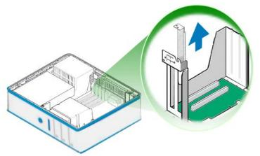
Step 6: Unscrew and remove the PCI slot cover from the computer case.
