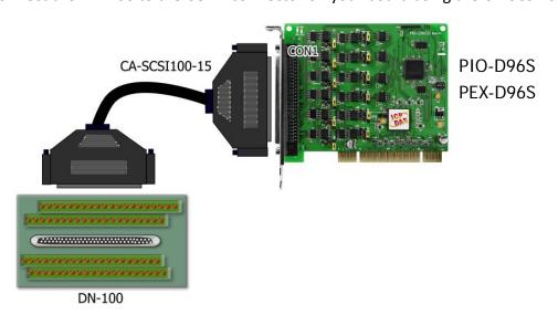
Step 2: Connect the Port0 (PA00 ~ PA07) with Port1 (PB00 ~ PB07).
