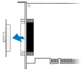
**Step 8:** Carefully insert your board into the PCI/PCI Express slot by gently pushing down on both sides of the board until it slides into the PCI connector.
