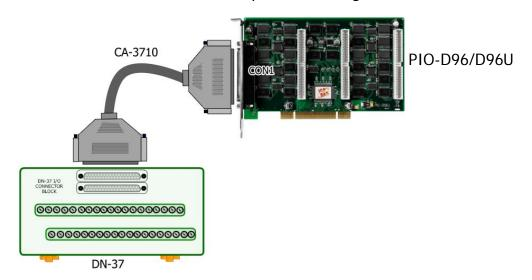
Step 2: Connect the Port0 (PAO ~ PA7) with Port1 (PBO ~ PB7).
