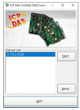
**Step 2:** Confirm that your board has been successfully installed in the Host system. **Note that the device number starts from 0**.
