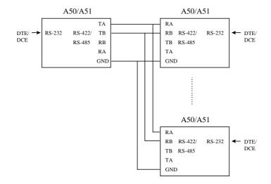
In the graph, TA, TB, RA and RB could be either from RJ-45 or Terminal Block. The settings of the switches for each A50 (or A51) are as follows:
