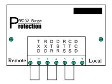
In the above graph, all the signal lines could be either from remote site RJ-45 or Terminal Block and shorted as shown.
