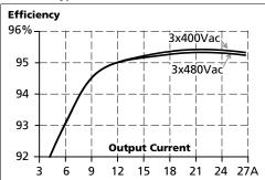
Fig. 12-3 Efficiency vs. input voltage at 36V,
