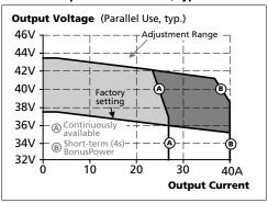
Fig. 6-4 Dynamic overcurrent capability, typ.
