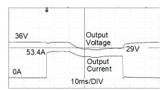
53.4A Peak load (resistive) for 50ms Output voltage dips from 36V to 29V.
