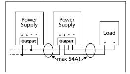
Fig. 15-2 Using distribution terminals
