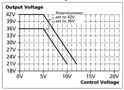
Fig. 10-2 Applying the control voltage
