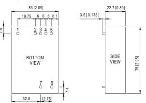
NOTE:PIN size tolerance 1.0  $\phi$  ±0.05mm
