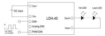
During PWM dimming operation, Io will change with the PWM duty (PWM Signal:  $1K\sim10KHz$ )
