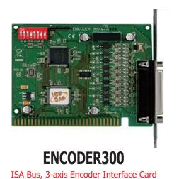
Accepts inputs from incremental or quadrature encoders
